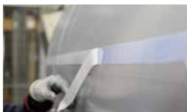
4th step: Remove the wide liner from the tape.
