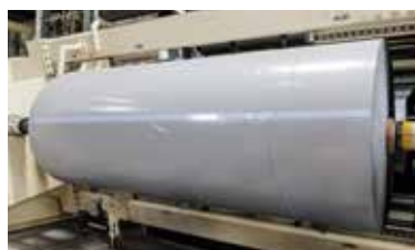
5th step: New web-material is ready for a flying splice.
