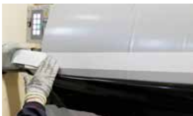
1st step: Apply the tape to the new roll.
